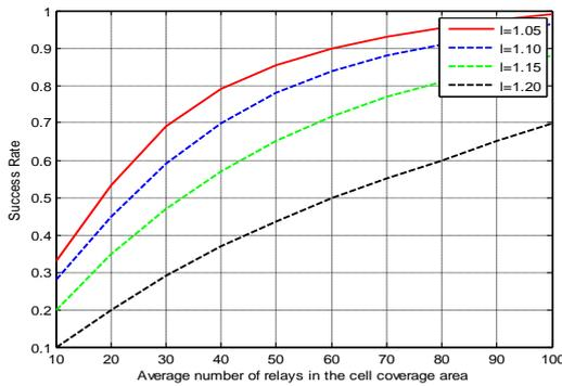
**Fig.3** The Probability of finding a feasible relay as a function of the average number  $N$  of relays in the base station coverage area, with path loss exponent  $\alpha = 3$  and  $\gamma_1 = \gamma_2 = 3$  dB
