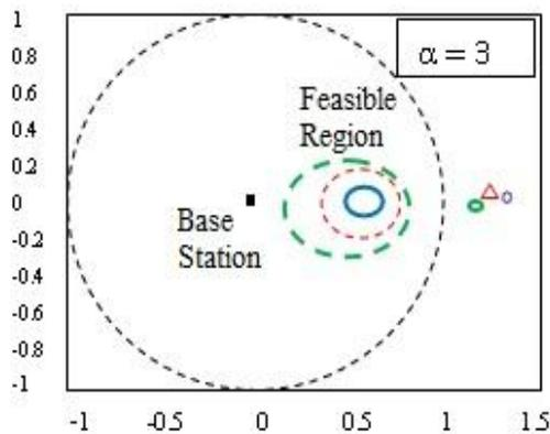
**Fig-2.** The feasible relay regions for  $\ell = 1.1, 1.2, 1.25$ , respectively, with path loss exponent  $\alpha = 3$  and  $\gamma_1 = \gamma_2 = 3\text{dB}$  and the length of the perimeter of the feasible region as
