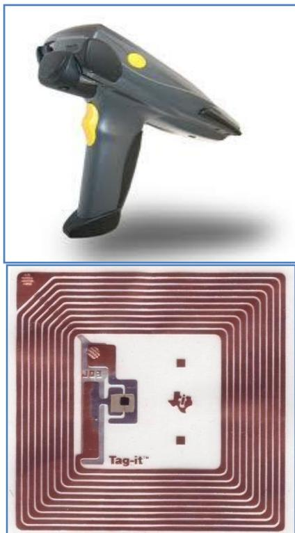
Fig-2: RFID Reader and RFID Tag[11]
