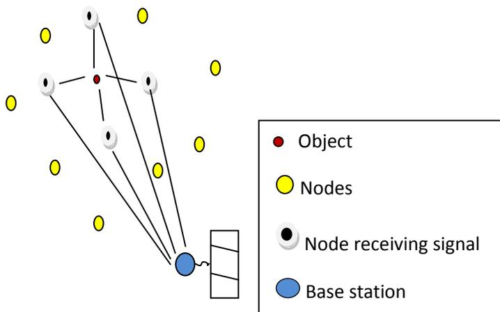
**Fig-1:** Locating objects in a Wireless Sensor Network [11]
