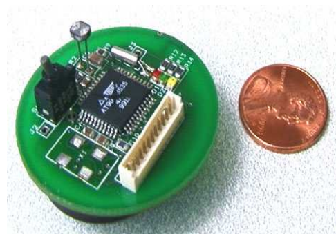
Fig-3 Smart Dust (Mote)
