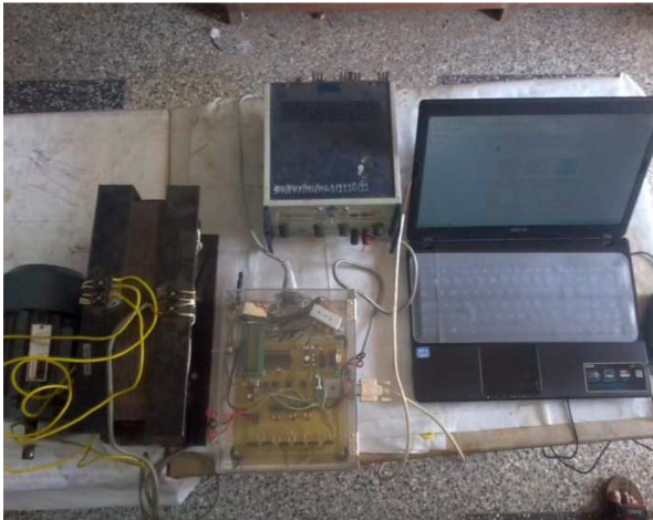
Fig.9 (a): Experimental Set Up of MATLAB Interface of Induction Motor
