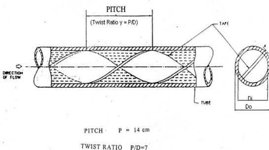
**Fig.2** Twisted tape inside a circular tube
