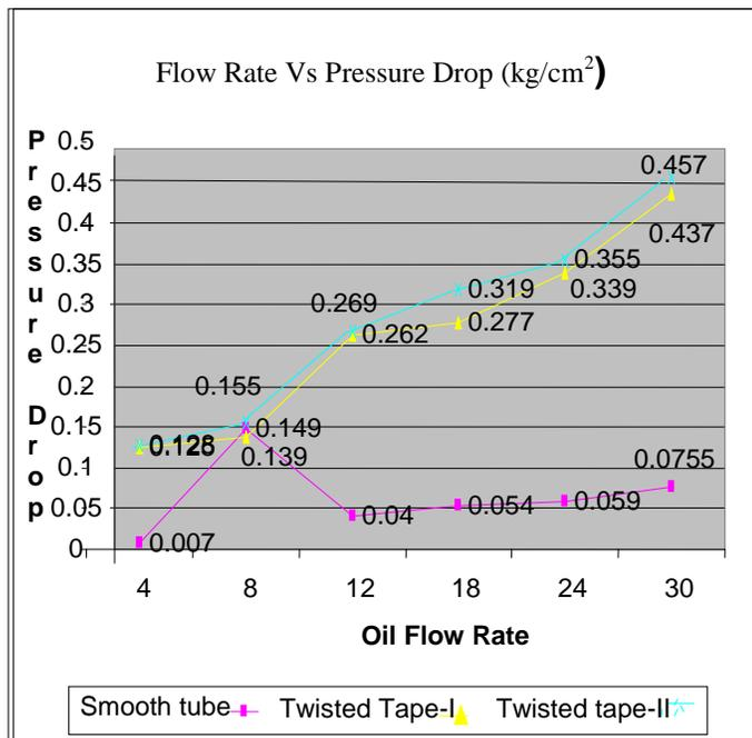
**c. Effect of Mass Flow Rate on Thermal Performance**
