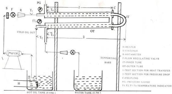
**Fig.1** Experimental Setup For Double Pipe Heat Exchanger
