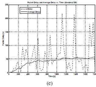
Fig 4: Scenario 2: Delay-insensitive routing. Packet delay and average delay vs. time for three source rates. (a): Source rate equal to 150 bps; (b): Source rate equal to 300 bps; (c): Source rate equal to 600 bps.
