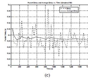
Fig. 5. Scenario 3: Delay-sensitive routing. Packet delay and average delay vs. time for three source rates. (a): Source rate equal to 150 bps; (b): Source rate equal to 300 bps; (c): Source rate equal to 600 bps.
