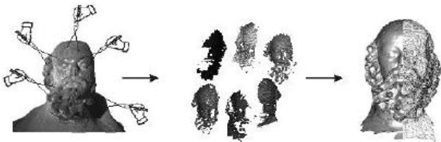
Figure 1: range images from different viewpoints have to be transformed into the same coordinate system.
