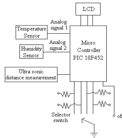
**Fig.1.** Block Diagram of the hand held device
