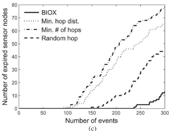
(a) Variance of sensor residual energies with increasing number of events. (b) Mean of sensor residual energies with increasing number of events. (c) Number of expired nodes with increasing number of events. includes the IDs of all frames previously received within a fixed time interval.
