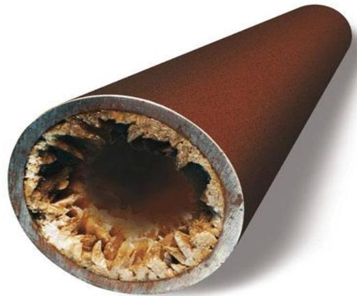
**Fig2:** Scaled oil and gas well production tubing.
