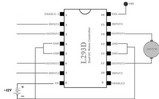
Fig 8 : Pin diagram of IC L293D
