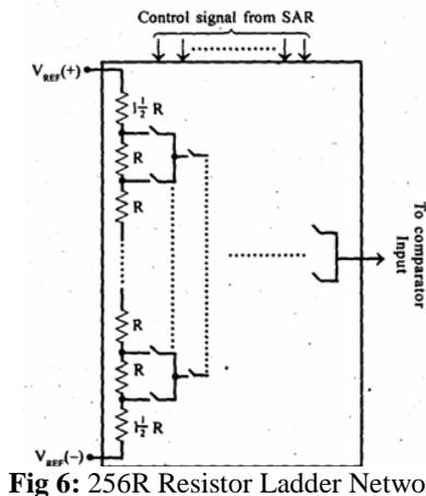
Fig 6: 256R Resistor Ladder Network
