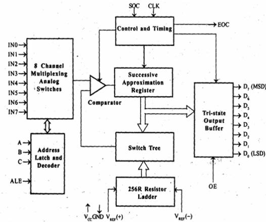
**Fig 5: Internal Block Diagram**
