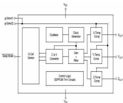
**Fig 3:** Functional Block Diagram of MMA7260QT
