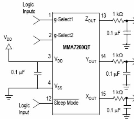
**Fig 4:** Accelerometer with recommended connection diagram
