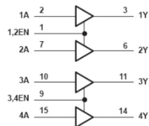
Fig 9 : Logic diagram of IC L293D
