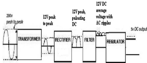
Fig 12 : Signal flow in Power Supply Unit
