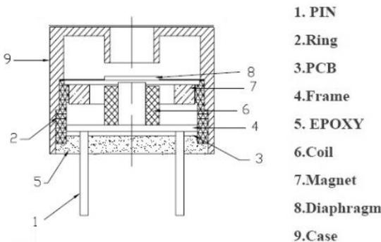
**Fig 10 :Internal Structure of Magnetic Buzzer**
