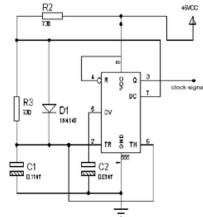
Fig 7: Circuit diagram of IC 555 timer operating as Astable multivibrator
