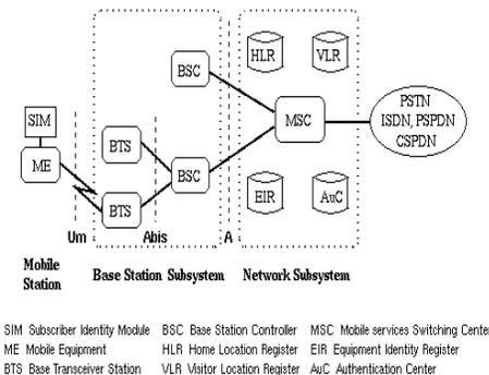
Fig 13 : Architecture of a general GSM network
