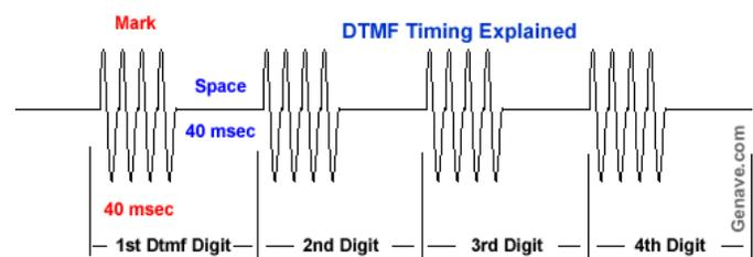
Fig3: DTMF Timing waveforms
