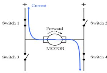
**Fig5:**H-Bridge Topology forward direction
