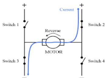
**Fig6:**H-Bridge Topology reverse direction
