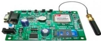
Fig-6: GSM modem
