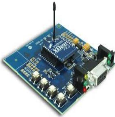
**Fig-2: Zigbee module**
