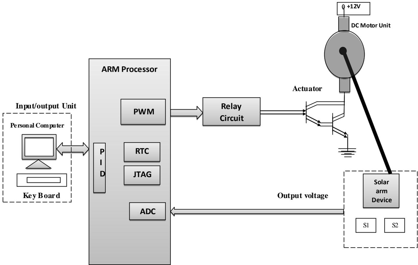
**Fig 2:** Block Diagram of the ARMProcessor based Solar tracking System
