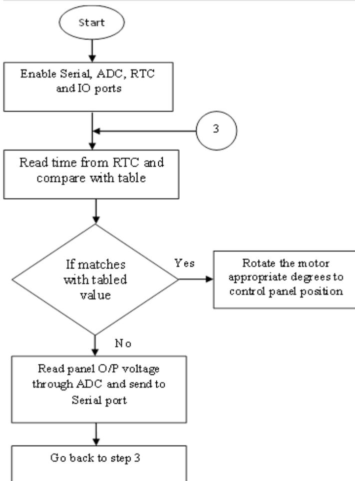
Fig: 3Flow-chart diagram for firmware development.
