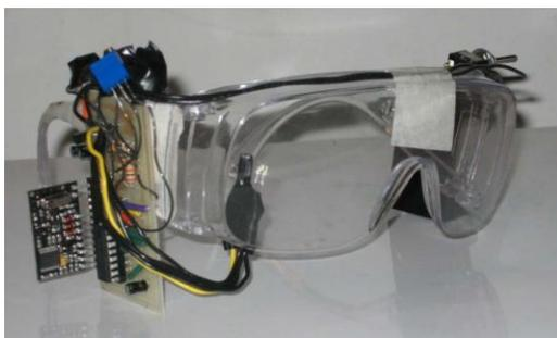
**Figure.2. Infrared Sensor Spectacles**
