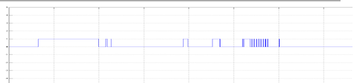
Gate pulses for Inverter in SHUNT APLC
