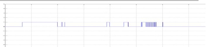
Gate pulses for Inverter in SHUNT APLC
