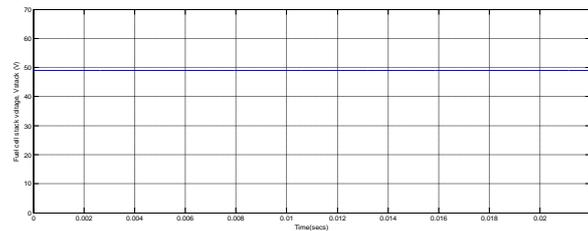
**Fig-11:** Waveform of fuel cell stack voltage which is input supply to asymmetrical dc-dc converter
