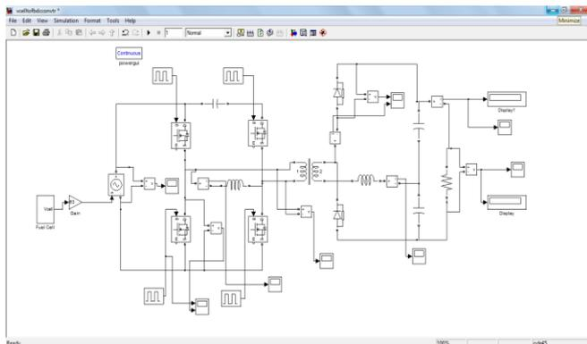
**Fig-10:** Simulated circuit diagram the Asymmetrical full bridge converter with fuel cell as dc source
