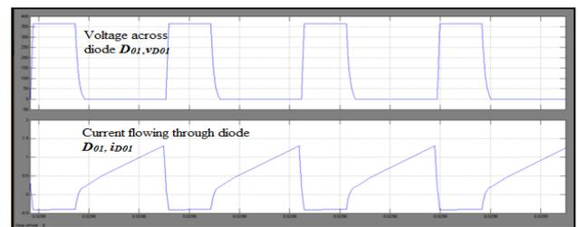
**Fig-17:** Waveforms showing voltage across and current flowing through, diode  $D_{01}$
