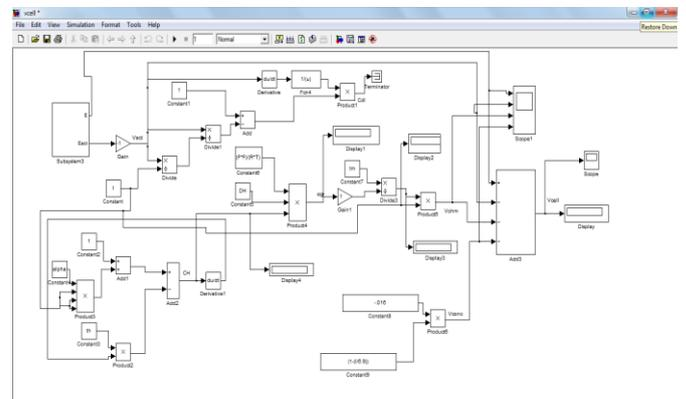
Fig-6: Matlab/Simulink model of PEM fuel cell
