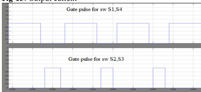
**Fig-14:** Waveform of driving pulses
