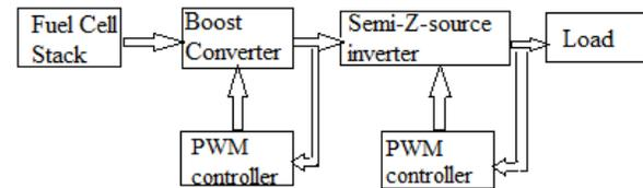
Fig. 1. Basic schematic block diagram for single phase FC system
