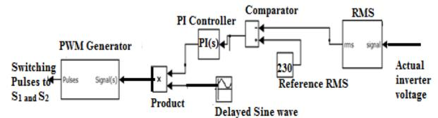
Fig 9. Control scheme for semi-Z-source inverter
