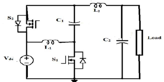
Fig.8 Semi-Z-Source converter
