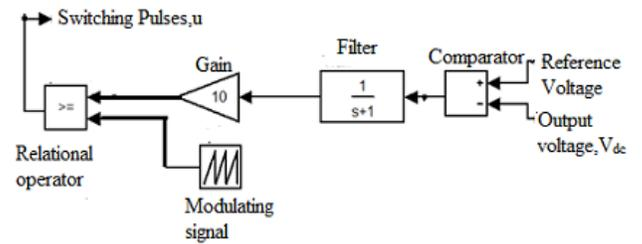
Fig. 4. Control scheme for dc-dc boost converter
