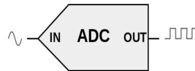
Figure 2: Analog to Digital converter
