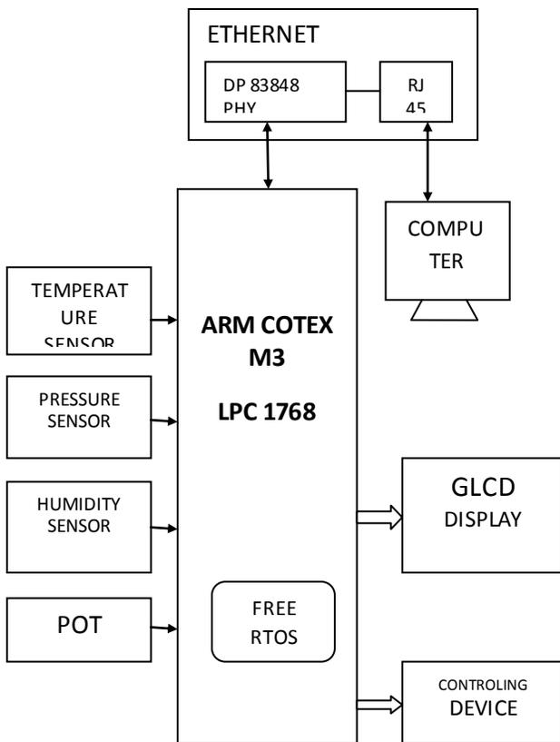
Figure 1: Block Diagram of Data Acquisition System
