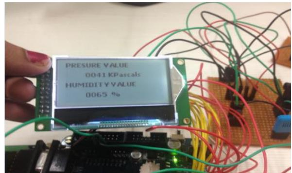
Figure 7: Initial sensor value on GLCD
