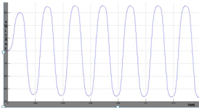
**Fig-19: The output voltage of PWM inverter**
