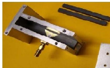
Fig -1 CBS slot antenna with non uniform biased ferrite material[2]
