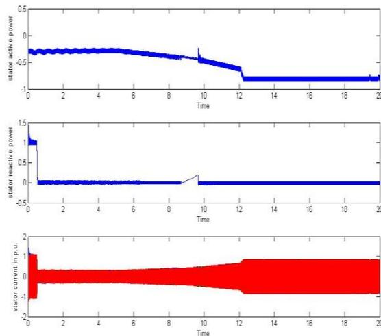
Figure 9: Stator active power, reactive power and current
