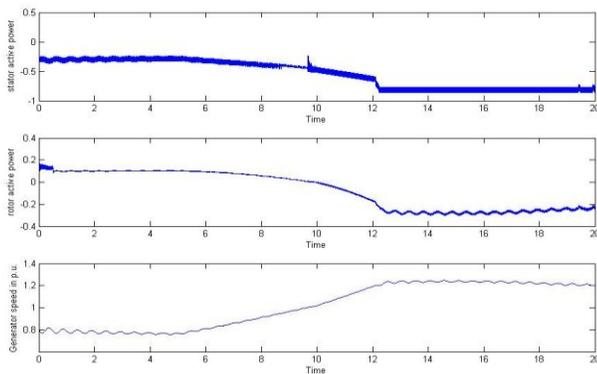
Fig. 10. Change in Rotor active power with speed
