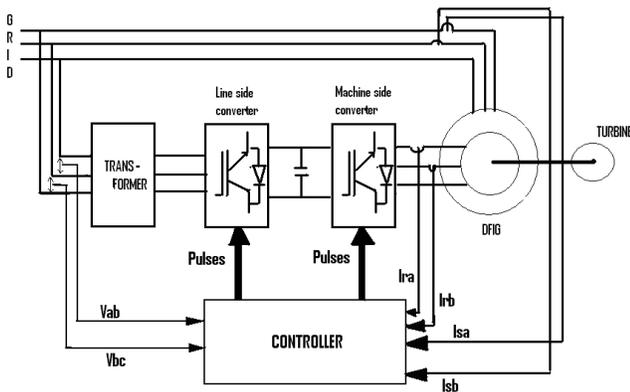
Fig. 2. Direct power control of DFIG
