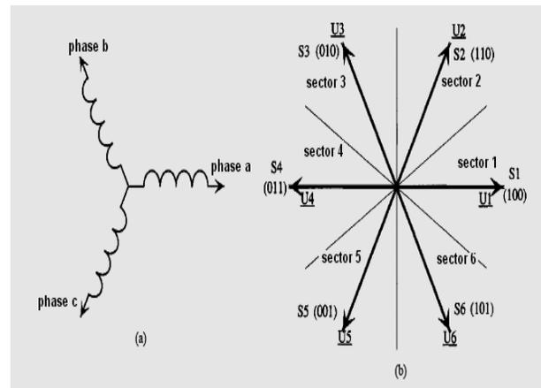
Fig. 3. (a) Orientation of the rotor winding in space with respect to which the voltage space phasors are drawn and (b) voltage space phasors.
