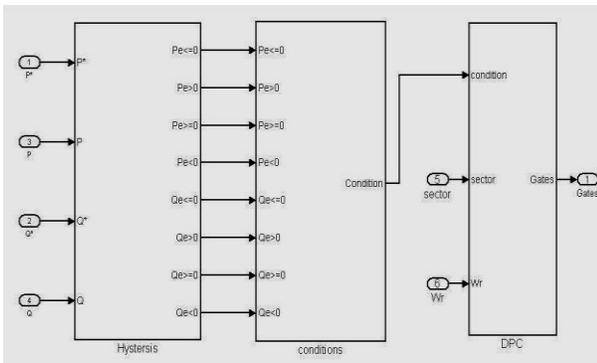
Fig. 4. Simulink model of direct power control scheme
