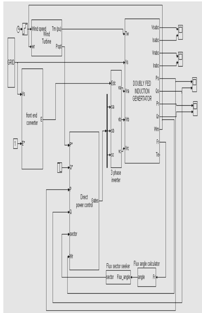
Fig. 5. Wind power generation by DFIG incorporated with DPC
