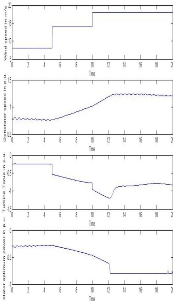
Fig. 6. Response of generator speed, mechanical torque and optimum power with change in wind velocity
