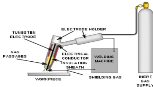
Fig: 1.2 TIG Welding Shielding Gas
