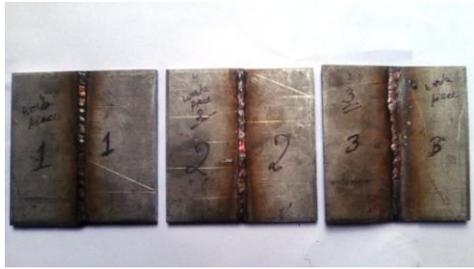
Fig. 1.3 Welded Samples 316 Stainless Steel
