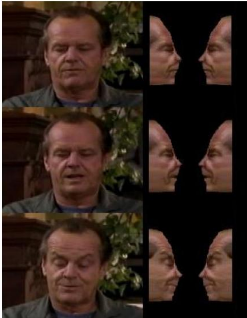
Fig 2: Video frames with profile views synthesized from a structure-from-motion analysis of the 70×80 pixel facial region. The profiles are mirror images except for differences in recovered 3D structure. The profiles on the left have poor structure between the mouth and nose because occlusion artifacts in the tracking were correlated with head nods. The profiles on the right have better shape from the tip of the nose to the top of the mouth because incomplete SVD was used to handle occlusions in the 3D reconstruction
