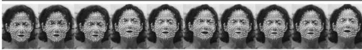
Every 300th frame from a 3000-frame sequence tracked via rank-constrained optical flow with incremental SVD. Dots are superimposed on the video by the tracker.
