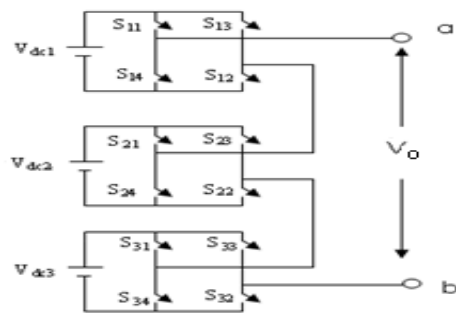
Figure 1: Single Phase 7 level Cascaded H-Bridge inverter
