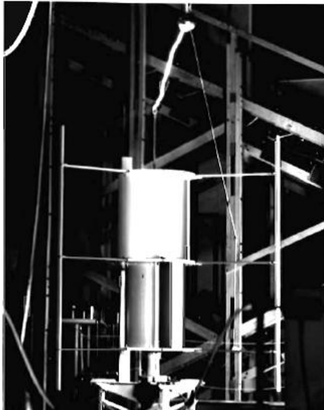
Fig- 9: The ERIGEN Turbine in Lighting strike test in a high voltage lab.
