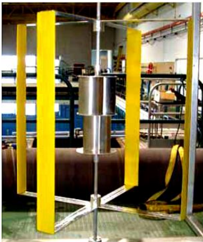
Fig- 12: Hybrid configuration of Darrieus and Savonius rotor
