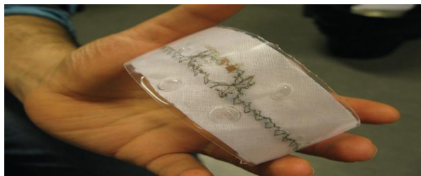
Fig. 10: PDMS Coated Embroidered RFID Tag
