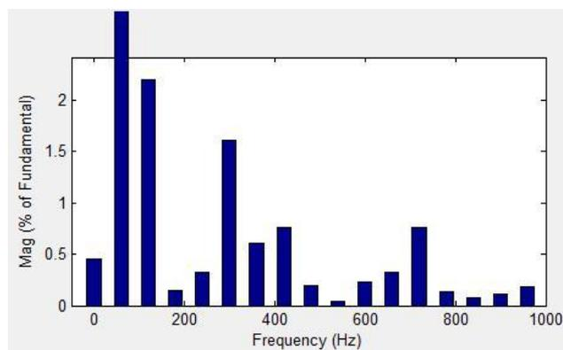
Fig. 16. Current harmonic spectrum at bus 11.
