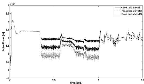
**Fig. 9. Utility grid2 active power at bus 2.**
