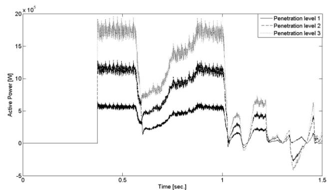
Fig. 5. Injected power by PV system at bus 11.
