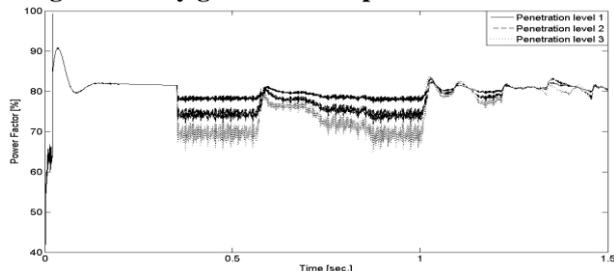
**Fig. 11. Utility grid2 power factor at bus 2.**
