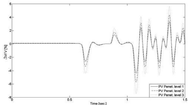
**Fig. 13. Measured flicker index at bus 6.**
