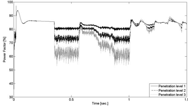
**Fig. 8. Utility grid1 power factor at bus 1.**
