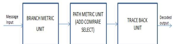
Figure:6 Block diagram of viterbi decoder.
