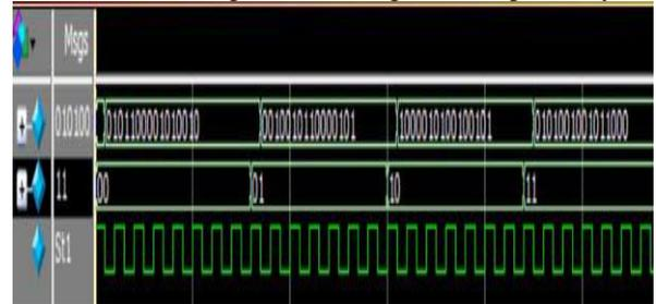
Figure.12. Simulation result of Branch Metric Unit.
