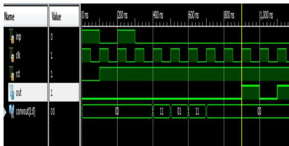
Figure: 15 Simulation result of modified viterbi decoder.
