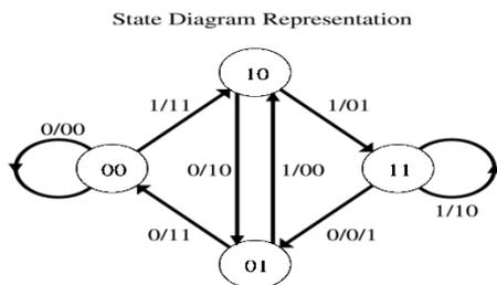
Figure: 3 State diagram of convolutional encoder.
