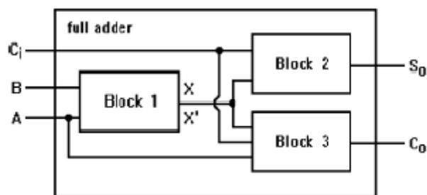
Figure 1 Full-adder cell formed by three main logical blocks.
