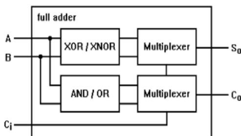
Figure 2 Alternative logic scheme for designing full-adder cells.
