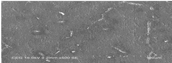
Fig-8:SEM micrograph of Mica 3% composition
