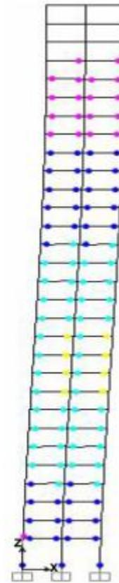
From distribution of hinges for 15-storey, it can be noticed that the plastic hinges were located at the fourth, fifth and sixth levels with severe failure. In addition, most of plastic hinges occurred in the beams, which satisfies the weak beam-strong column criteria. Moreover, critical section was located on the columns of the tenth floor, as for these columns the load was released which is an indication for the near failure for the soft storey in building.
