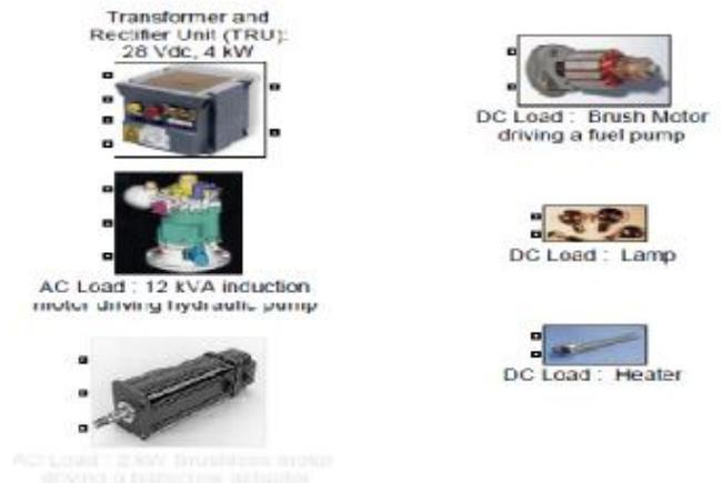
Figure 1 Different type of loads used in Aircraft [37]
