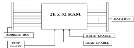
Fig. 2 Block Diagram Of 2K \* 32 bit SRAM
