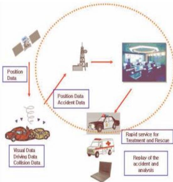
The car black box is used to detect various information such as driving data, data of collision and the data of previous position of the vehicle and the position of vehicle after the accident. This information will be useful to examine the accident easily and to solve the problems associated with car accident.
