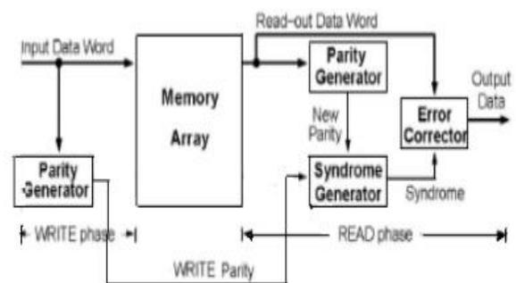
Fig. 3 Integration of SRAM with EDAC unit
