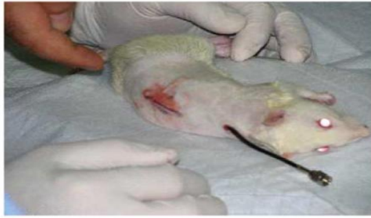
Fig 1.5: Testing of an implantable patch antenna inside animal tissue: antenna surgically implanted into a rat.
