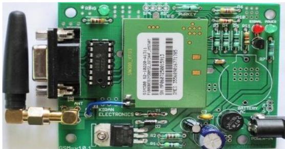
GSM modem gives capability to send SMS without any mobile operating system. SIM can be read with MCU and can be used to send SMS by micro controller. Hence a GSM modem was employed, its main function here was when the parameters are over threshold limits it sends a text message to predefined contacts about the situation of the person thus alerting them to proceed for further actions.
