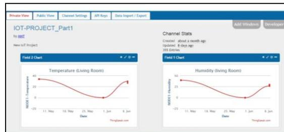
Above figure shows the graphical representation of the data which is coming indirectly from the slave nodes. This graphical data is formed from the continuous stream of data which is store on the Thing speak cloud. This data can be parsed into any format and is easily available for viewing on website as well as hand held devices platform.
