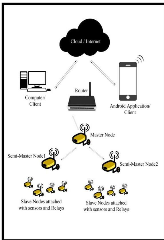
As Shown above in the figure, we have slave nodes which are transmitting and receiving the data for sending the sensor data or receiving the data for operating the relays and appliances. The clients are the user who are constantly monitoring or controlling the sensor network. The Cloud is the data center where the data is stored securely.
