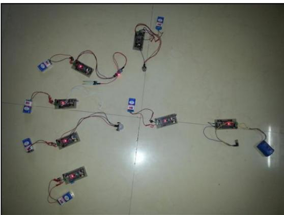
In the above figure we can see a system where five slave nodes are connected to a semi master node and the semi master node is connected to the master node which is directly connected to the internet cloud through a router.
