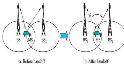
Figure 1.1 Hard handoff between the MS and BSs.
