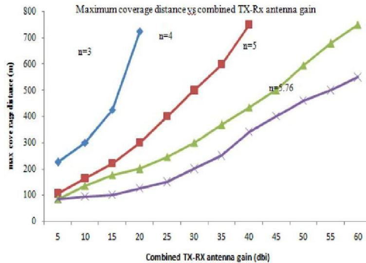
Fig. 7: Maximum coverage distances at 28 GHz with 119 dB maximum path loss dynamic range
