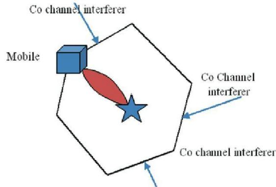
Fig. 3: Use of highly directional receiver antenna system
