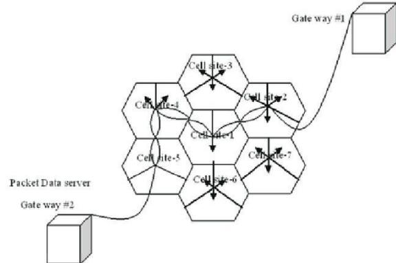
Fig. 4: Cell systems may use steerable antenna Array
