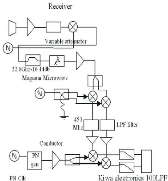
Fig. 6: RX for the mm wave measurement at 28 GHz
