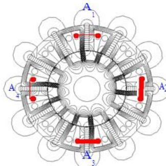
Fig. 5. Flux distribution at the  $d$ -axis position of phase  $a$ .
