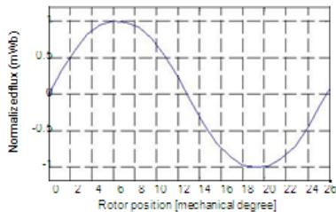
Fig. 3 Coil-flux linkage in one phase
