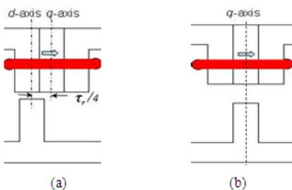
Fig. 4. Rotor at (a)  $d$ -axis position where the coil-flux linkage is maximum,
