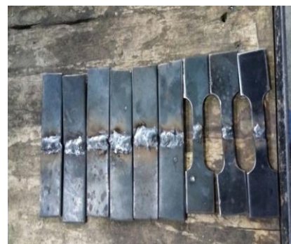
Final Welded Pieces
