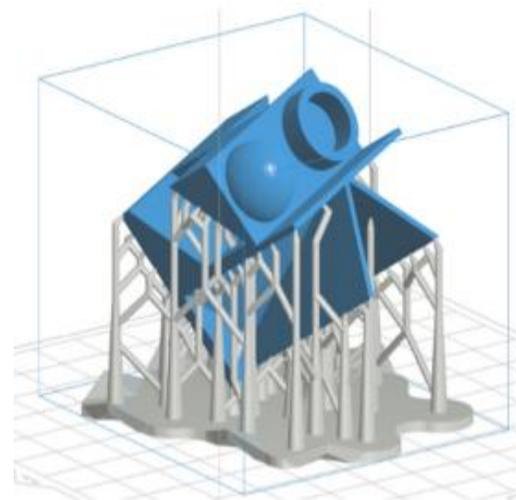
Fig. 2. Build direction of SLA sample in printer.
