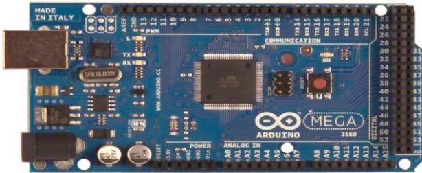
Fig-4.2: Arduino Mega
