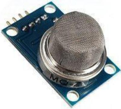
Fig-5.1.1: Mq2 arduino gas sensor
