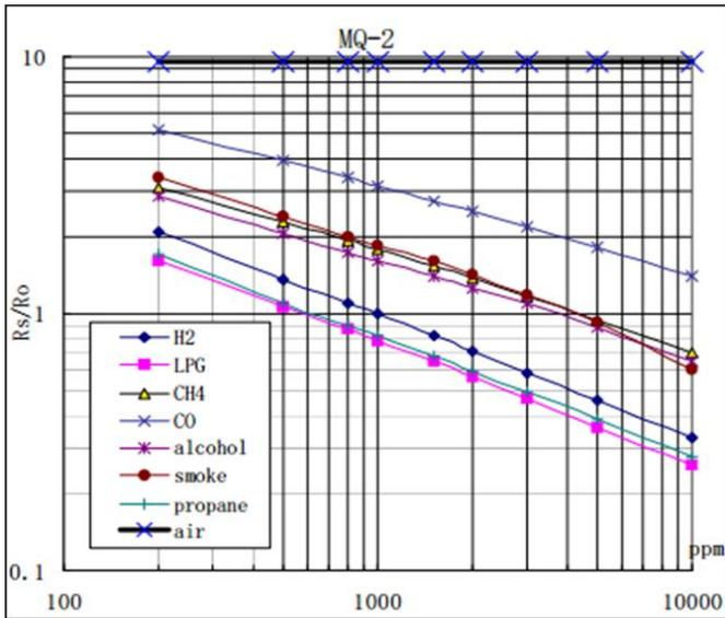
Fig-5.1.2: Sensitivity Characteristics
