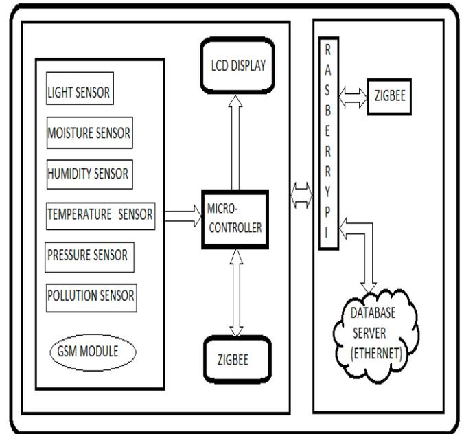
**Fig-4: The overall system architecture**
