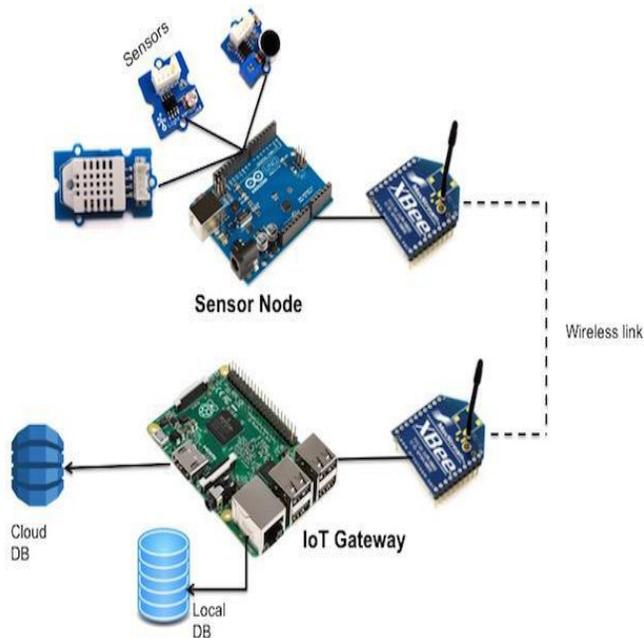
**Fig-7.1: Overall system design**
