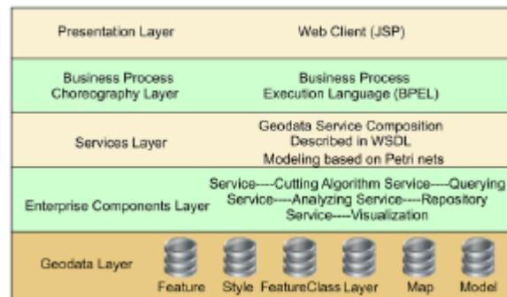
FIGURE 3. Implementation architecture of geodata service composition web application.
