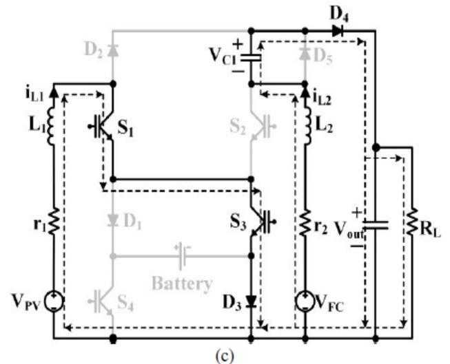
Fig. 2. Current-flow path of operating modes in first operating state. (a) Mode 1. (b) Mode 2. (c) Mode 3.
