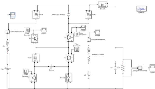
**Fig. 6 Matlab Simulink for proposed converter**
