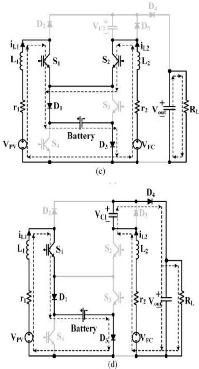
Fig. 3. Current-flow path of operating modes in third operating state. (a) Mode 1. (b) Mode 2. (c) Mode 3. (d) Mode 4.
