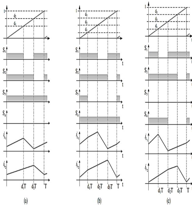
Fig. 4. Switching pattern for three states. (a) First state. (b) Second state. (c) Third state.
